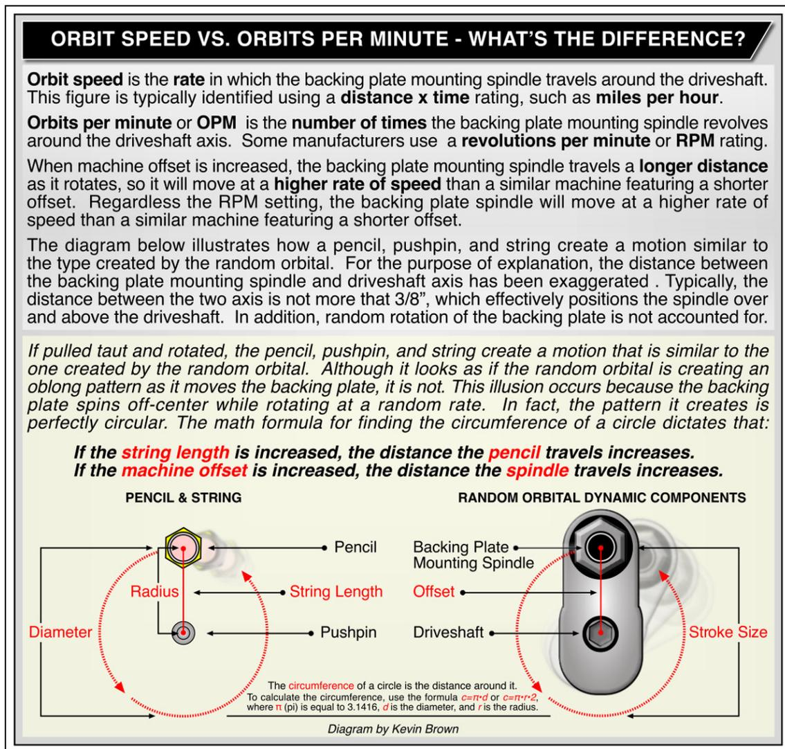
A majority of random orbital machines use a stroke diameter that measures somewhere between 1/8" to 5/16" (approximately 3.0mm-8.0mm). It is generally accepted that a smaller stroke leaves a more refined finish, but reasoning and experience tell a different story.
