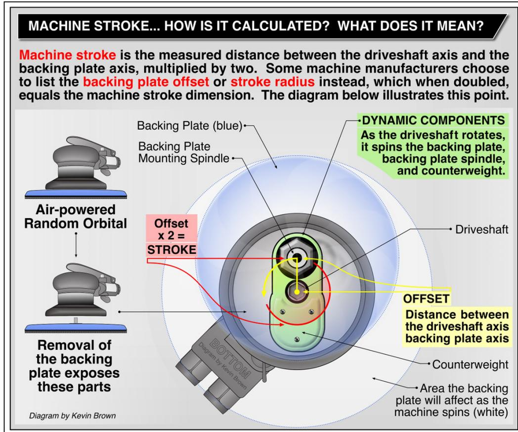
Machine manufacturers also refer to machine offset using terms such as backing plate offset, stroke radius, and stroke diameter. Regardless the terminology, these terms are all identifiers of the machine's movement.
