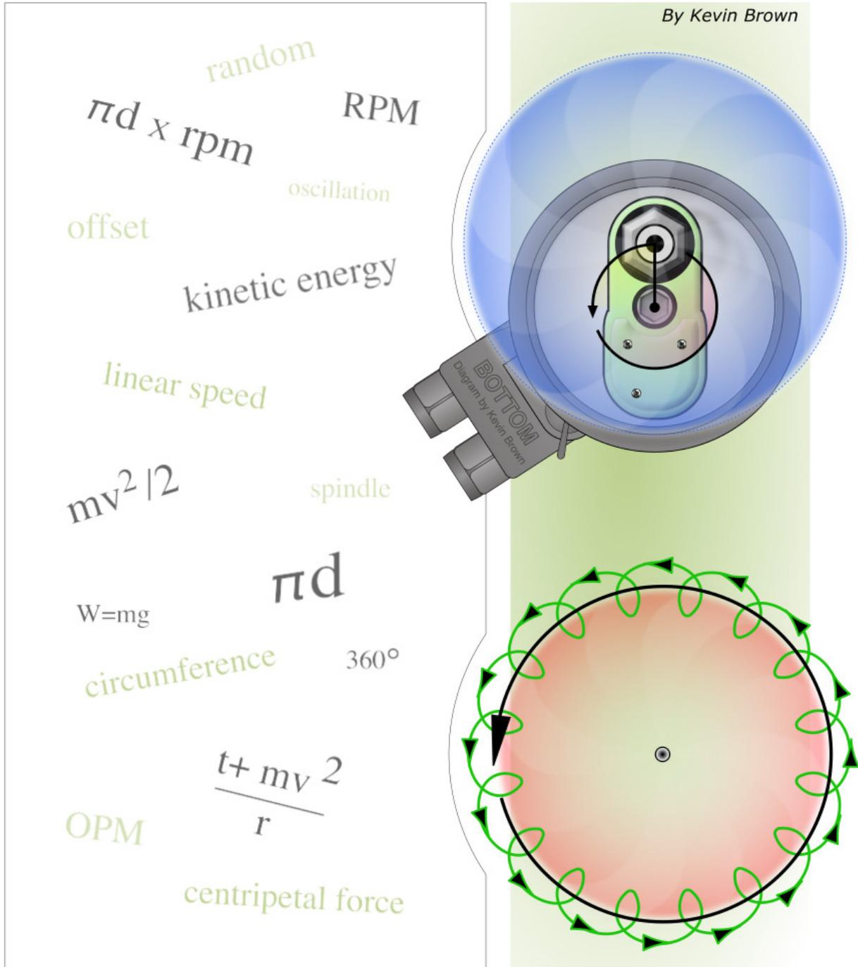
**Machine stroke** is a term that identifies the diameter of the path the backing plate travels as it circumnavigates the driveshaft. Since the machine's driveshaft is rarely level with the backing plate, machine stroke actually refers to the driveshaft axis and the *backing plate* or *backing plate mounting spindle* axis. The diagram below illustrates this point:
